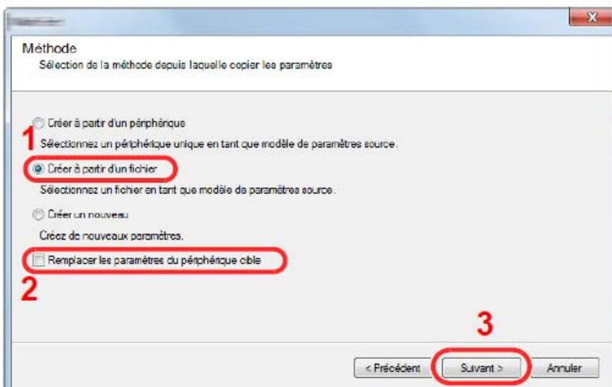
Selecting the [Replace Target Device Settings] check box will overwrite the machine's address book from entry n° 1.
