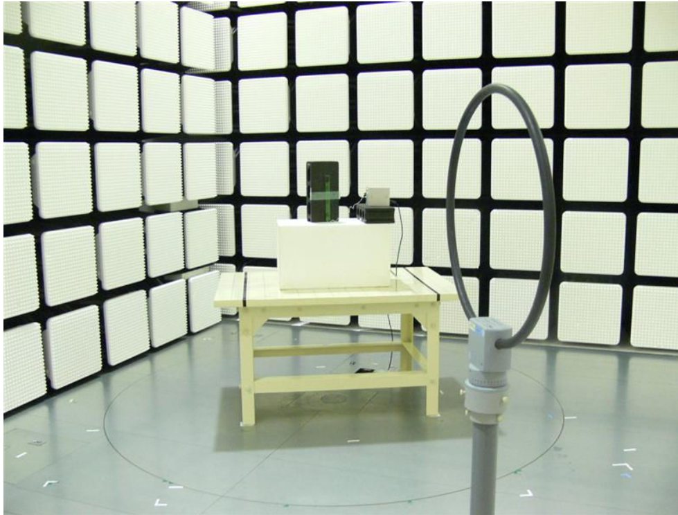
Photograph 4: Set-up for Radiated Spurious Emissions below 30MHz
