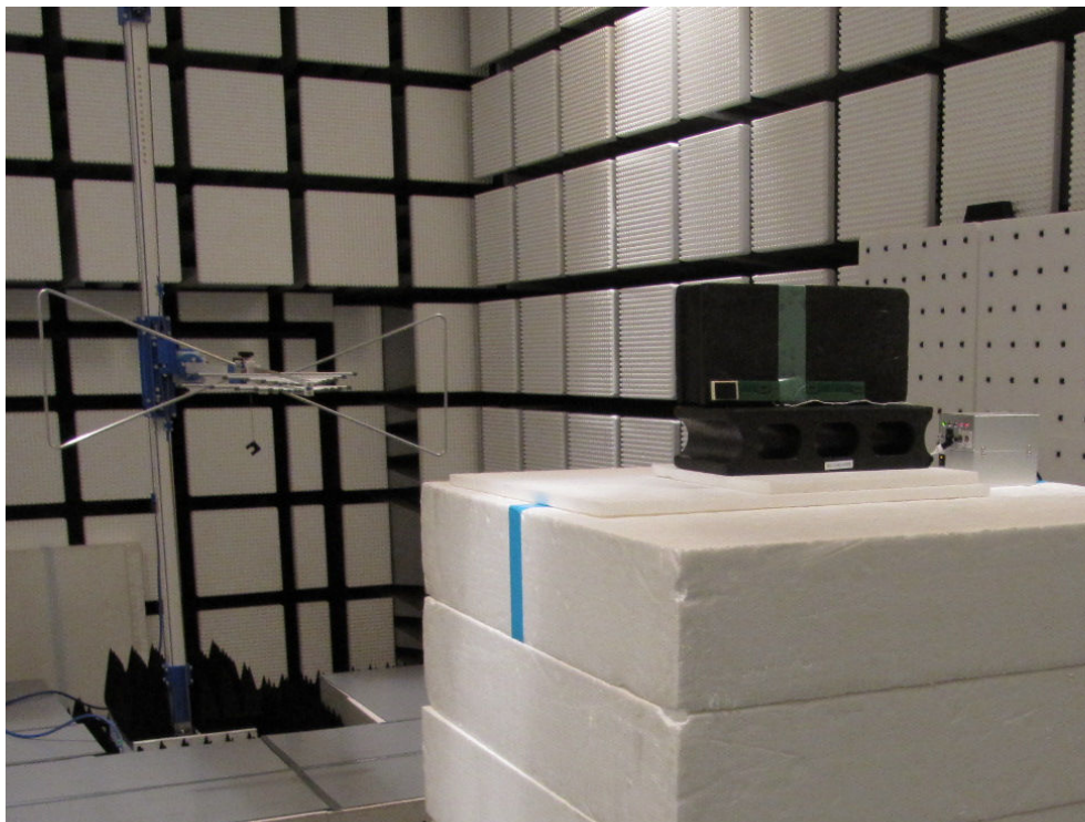
Photograph 5: Set-up for Radiated Spurious Emissions above 30MHz
