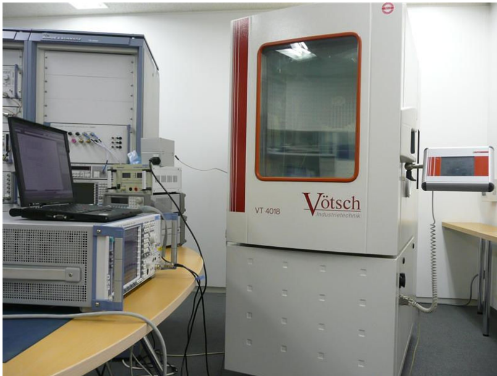
Photograph 2: Set-up for Antenna Port Conducted Measurements, General View
