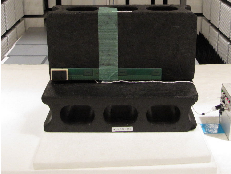
Photograph 6: Set-up for Radiated Emissions, EUT Configuration X-Axis
